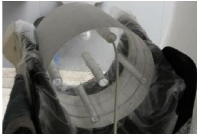
Figura 2, newborn head phantom placed in the gantry isocenter.
