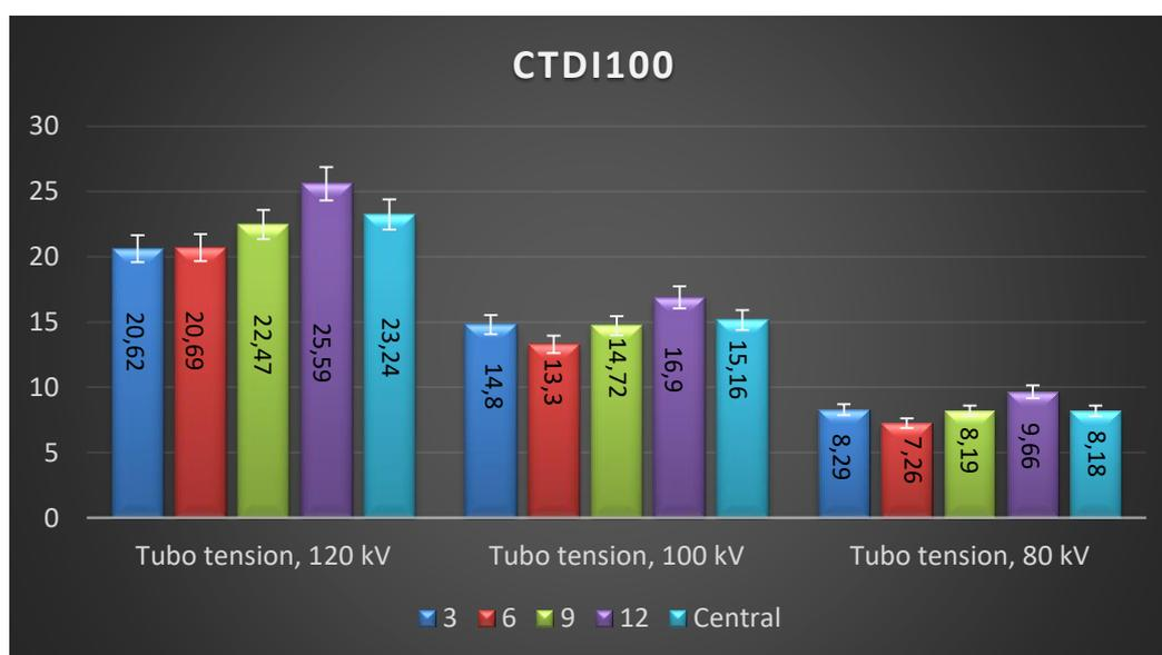
Figure 4, Mean values of  $C_{k,100}$  measurements for NB phantom
