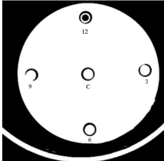
Figura 3, axial section of the simulator object with the identifications of the apertures with the pencil chamber positioned in the aperture 12.
