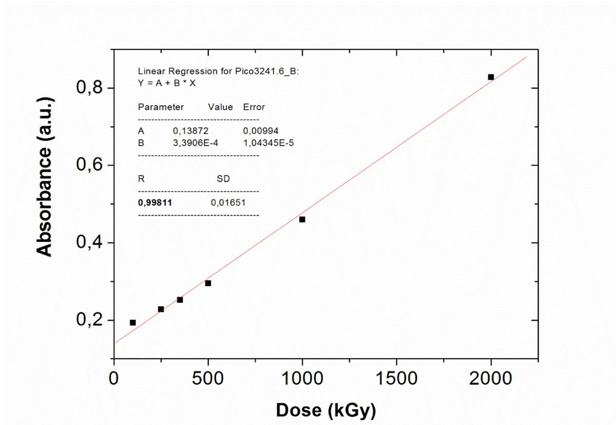
**Figure 6:** Plot of the absorption peak intensities at  $3241\text{ cm}^{-1}$  as a function of the delivered dose, taken from Fig. 4. The linear regression data are displayed in the inset, with the correlation coefficient of 0.9981.
