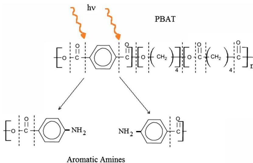
**Figure 5:** Structure of PBAT and chemical bonds that could be broken by gamma radiation, provoking chain scission. Photoluminescent aromatic amines could be formed by linking a hydrocarbon ring with an  $\text{NH}_2$  molecule
