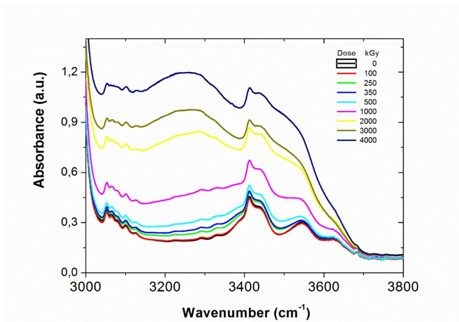
**Figure 4:** FTIR spectrograms of Ecoflex films irradiated with gamma doses ranging from 0 to 4.0 MGy in the 3,000 to 3800  $\text{cm}^{-1}$  wavenumber range.
