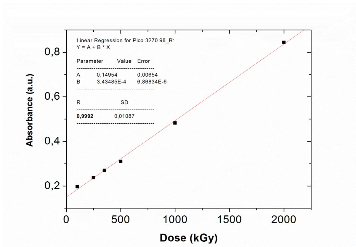
**Figure 7:** Plot of the absorption peak intensities at  $3271\text{ cm}^{-1}$  as a function of the delivered dose, taken from Fig. 4. The linear regression data are displayed in the inset, with the correlation coefficient of 0.9922.
