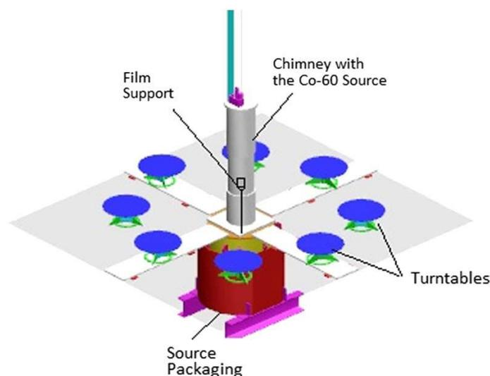
Schematic drawing—irradiation setup.
