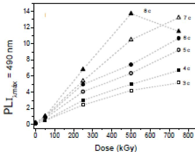
**Figure 3:** PL output as a function of gamma doses for samples with with 3 layers (38  $\mu\text{m}$  thick), 4 layers (49  $\mu\text{m}$ ), 5 layers (61  $\mu\text{m}$ ), 6 layers (75  $\mu\text{m}$ ), 7 layers (106  $\mu\text{m}$ ) and 8 layers (130  $\mu\text{m}$ ), produced by using the *wire-bar coating* technique.
