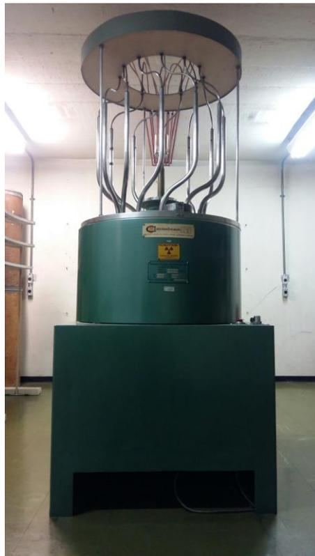
**Figure 1. *Gammabeam-650*<sup>®</sup> irradiator from CENA/USP used to sterilize the flies as pupae 48 h before the emergence of the adults.**
