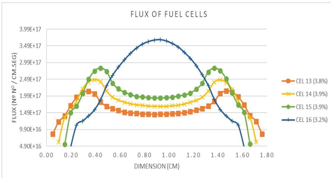
**Figure 7: Relation of flux between all fuel cells simulated.**
