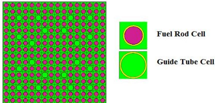
**Figure 1: Reference (16x16) typical fuel assembly.**
