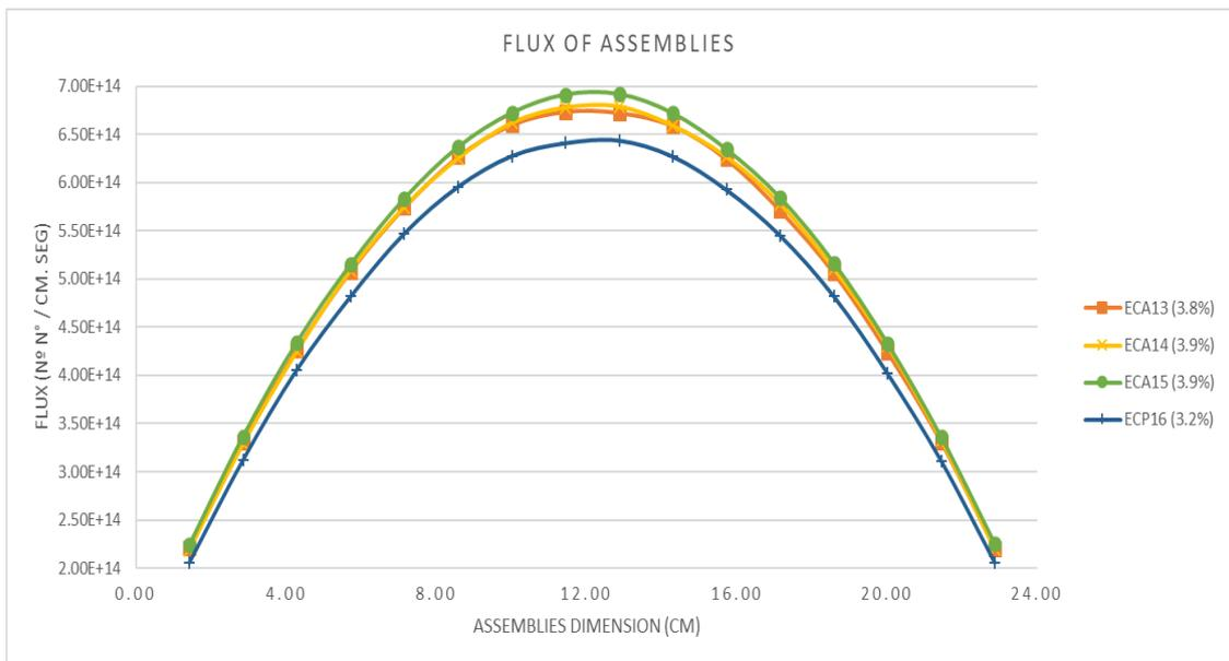
**Figure 6: Relation of flux between all assemblies simulated.**
