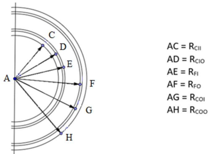
**Figure 3: Radius of Annular Fuel Rods worked in the research.**
