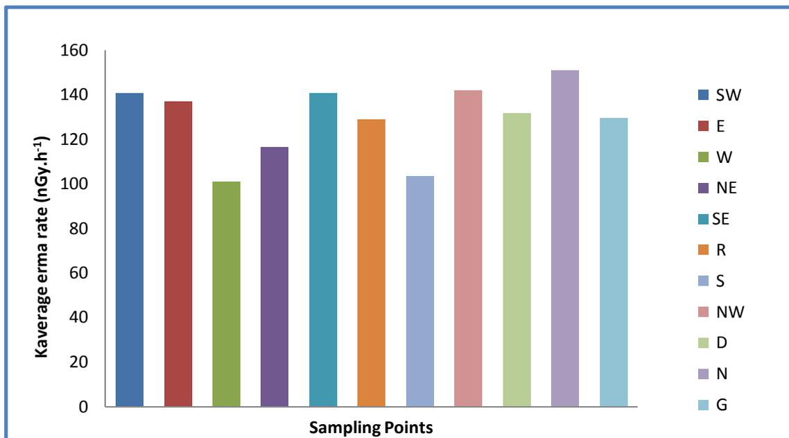
**Figure 2: Measurements of environmental gamma radiation level using TLD.**
