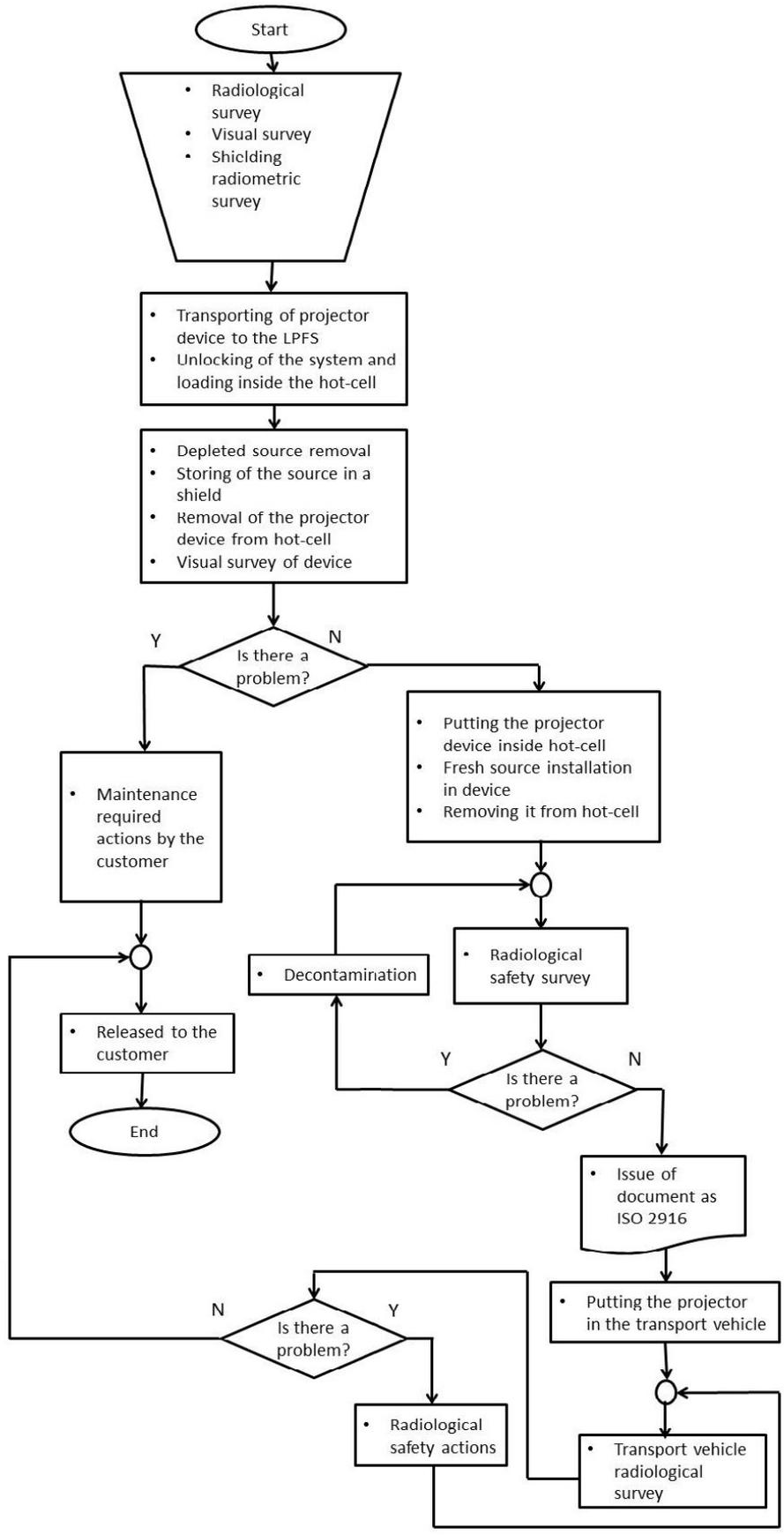
**Fig. 6: Changing a source of exposure device**
