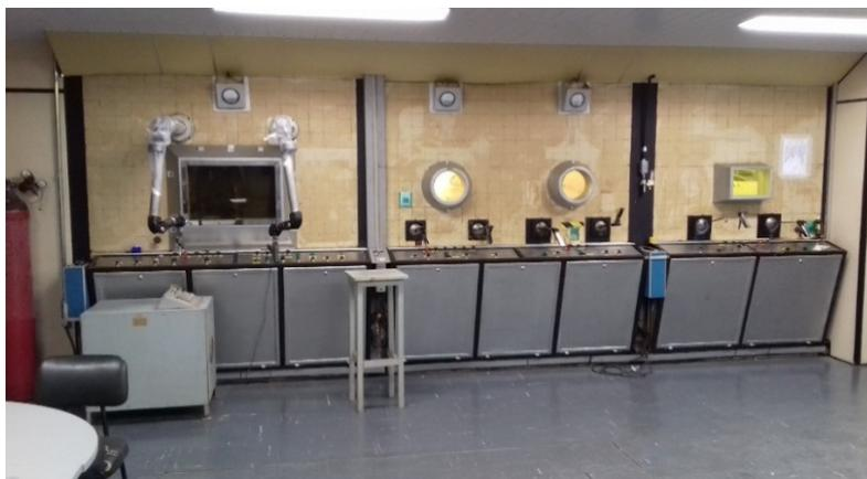
**Fig. 2: Hot-cells inside the LPFS -Zone 1**
