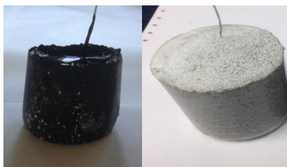
Figure 4. The sample of bitumen (left) and bitumen encapsulation in cement paste or in mortar (right)
