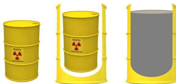
Figura 3. Encapsulation of drums containing bituminized radioactive waste.
