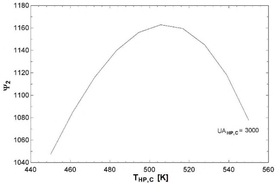
**Figure 6: Variation of  $\psi_2$  in comparison with the cold heat pipes' temperature of operation.**
