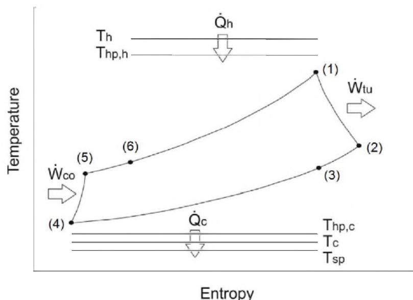
**Figure 3: T-s diagram for a CBC with recuperator – Adapted [5].**
