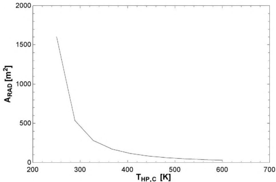
**Figure 4: Variation of the radiator's area when compared with the cold heat pipe's evaporator temperature.**
