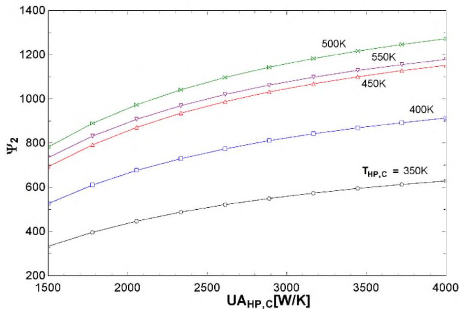
**Figure 10: Optimal temperature range of operation of the CBC's cold heat pipes.**
