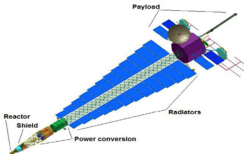
**Figure 1: Conceptual nuclear powered spacecraft design with the proposed CBC – Adapted [3].**
