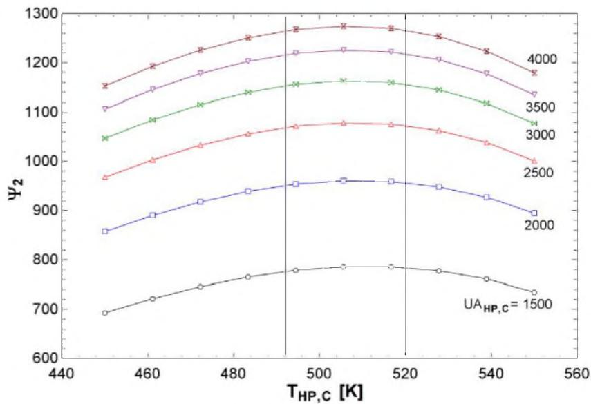
**Figure 9: Optimal temperature range of operation of the CBC's cold heat pipes.**
