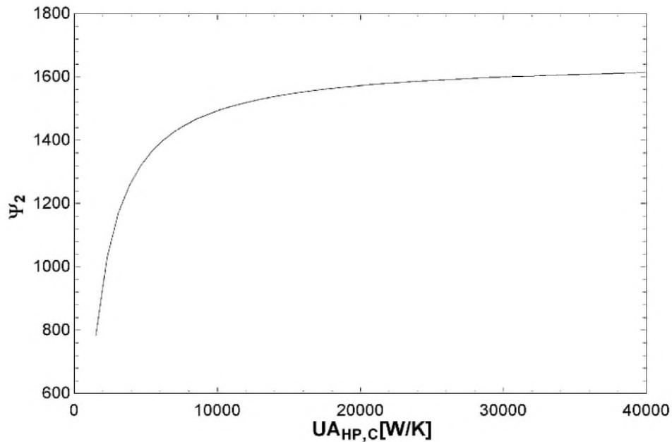
**Figure 7: Variation of  $\psi_2$  when compared with the cold heat pipes conductance coefficient.**
