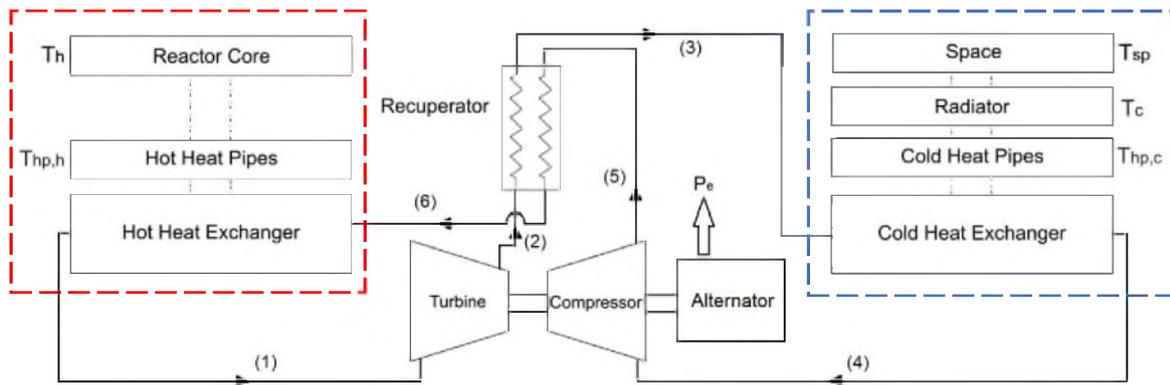
**Figure 2: Basic components of proposed CBC with recuperator.**
