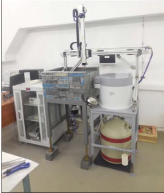
Fig. 6. Automation system for measurement of spectra
