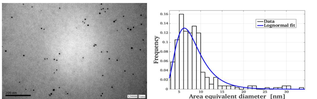
Figure 1.- TEM image of the silver nanoparticle synthesis product (left) and particle size distribution (right).
