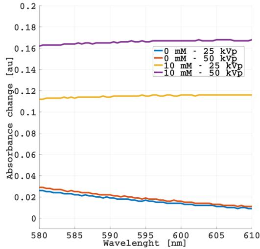
Figure 2.- Absorption spectrum for silver nanoparticles infused Fricke gel samples and standard BFGD.
