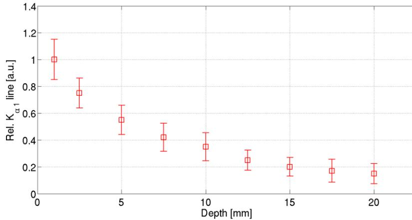
Figure 4.- Relative intensity (normalized at 1 mm depth) of detected K-alpha line positioning the 2% w/w AgNP-infused Fricke gel dosimeter at different water-equivalent depths.
