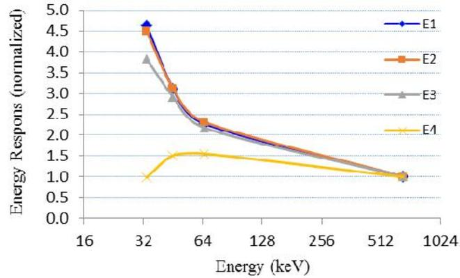
**Figure 5:** Response of OSLDs-p,e elements as a function of energy
