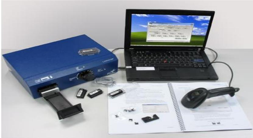
**Figure 2:** The Microstar reader connected to a computer
