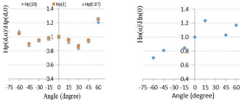
**Figure 3:** Angular dependence of OSLDs (left: for OSLDs-p,e and right: for OSLDs-n,p,e)
