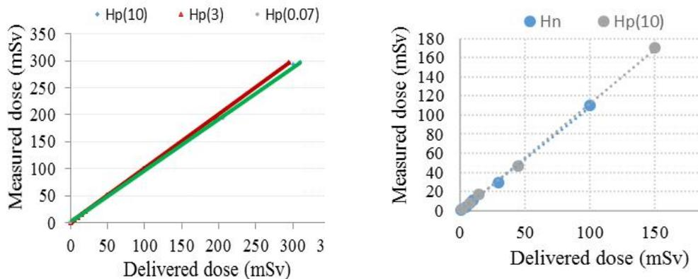
**Figure 4:** The linearity of OSL and OSLN dosimeters
