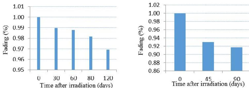
**Figure 6:** The fading of OSLDs after irradiation (left: for OSLDs-p,e and right: for OSLDs-n,p,e)
