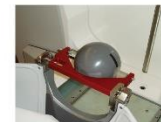
Figure 4: Setup of the PMMA phantom with the eppendorf tube for the LGK irradiation
