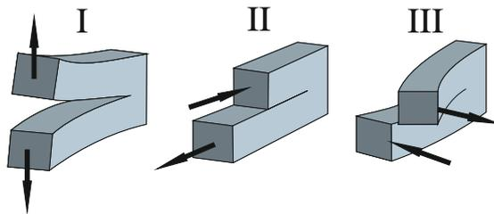
Fig. 2 Fracture modes (I-Opening, II-Sliding, III-Tearing)
