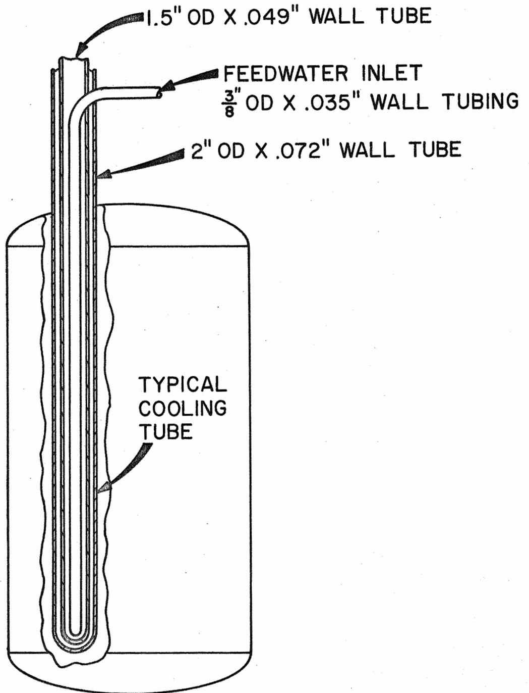
FIG. 2. COOLING TUBE ARRANGEMENT IN DRAIN TANK
