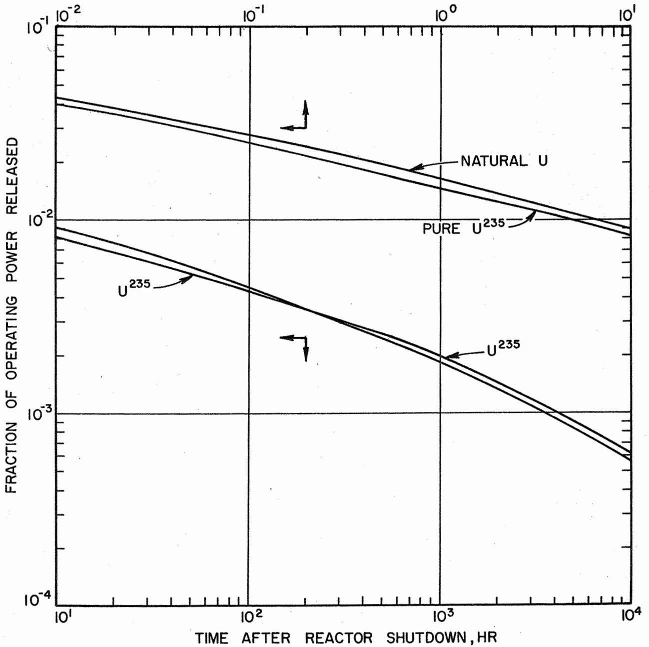
FIG. I. AFTER-HEAT RELEASE FROM NATURAL URANIUM AND U<sup>235</sup> vs TIME FOR INFINITE IRRADIATION PERIOD. REPLOTED FROM ANL 4790
