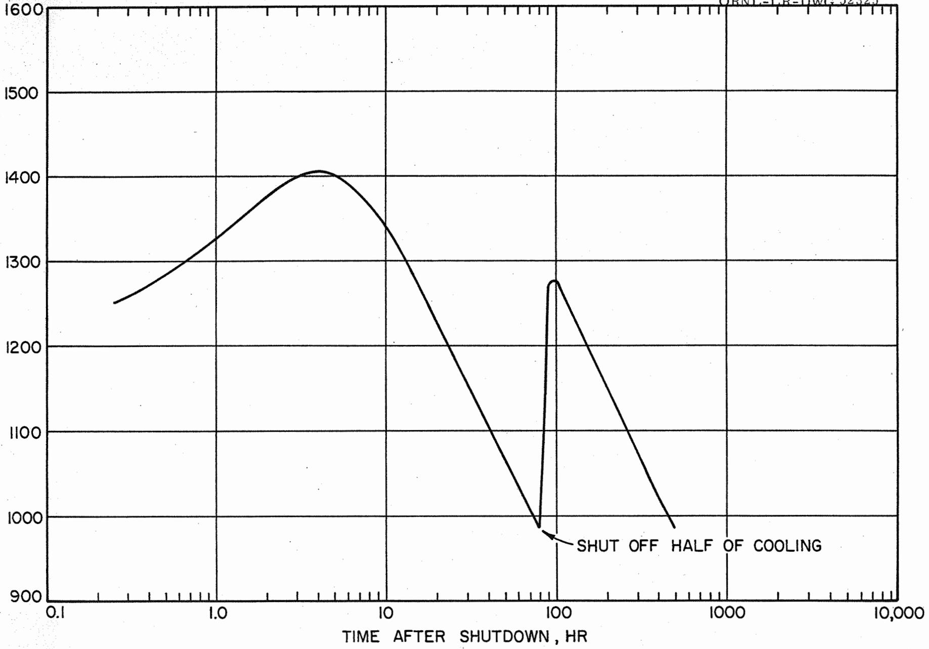
FIG. 4. TIME - TEMPERATURE BEHAVIOR OF MSRE DRAIN TANK HAVING COOLING CAPACITY RATED 100 KW AT 1300°F.
