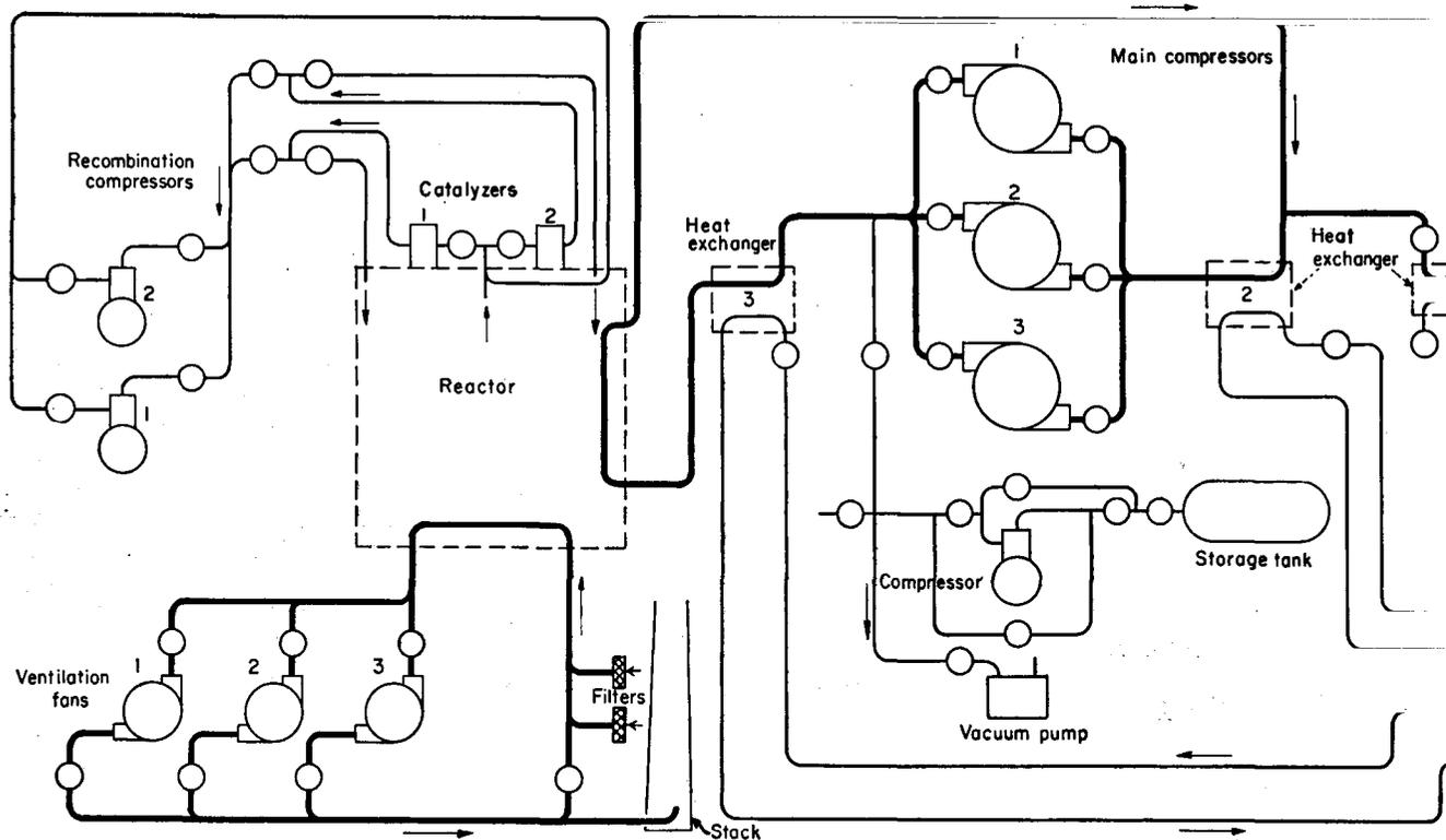
1. **PILE COOLING CIRCUIT** (heavy lines) uses two blowers, with third as standby, drives gas towards reactor at maximum absolute pressure of 170 lb/in<sup>2</sup> for nitrogen. Each blower handles flow of 30–35 metric tons of gas per hour, uses 400 kw. Exchanger 3 cools gas to 20–30° C before entering reactor. Gas leaves reactor at about 70° C (higher temperatures will be possible shortly), gives up its heat to exchanger 2 (exchanger 1 not used at
